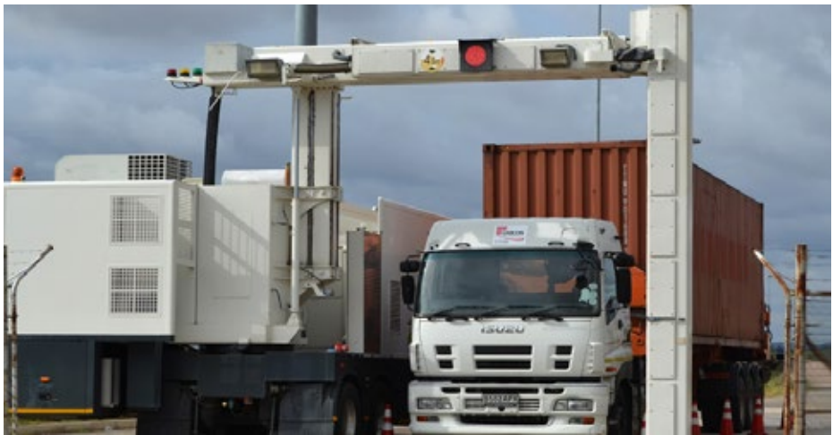
large-scale X-ray scanning equipment acquired by the Botswana Unified Revenue Service (BURS) for border posts to detect contraband like drugs, weapons, or smuggled goods. Photo Credit Botswana Unified Revenue Service (BURS)
